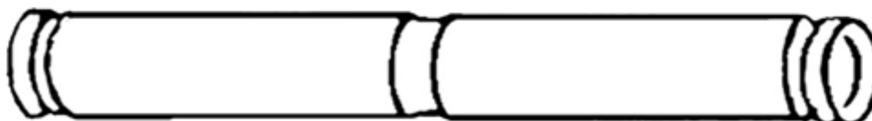
# 9 - 230 ROD SPLICER, USE WITH 3/8" (10mm) RODDING.
